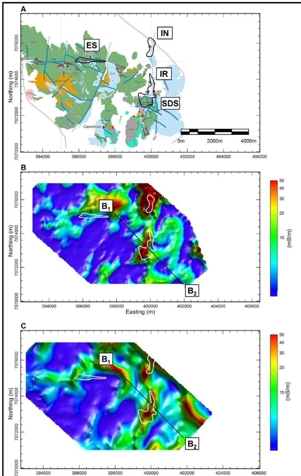
**Figure 9:** Property Geology after Daroch (2011) showing deposit outlines (A), 300 m depth below surface section through 1D inversion of 25 Hz VTEM (B), 3D inversion of 25 Hz – 600 Hz ZTEM (C). Black line represents the extent of section B<sub>1</sub> to B<sub>2</sub>.
