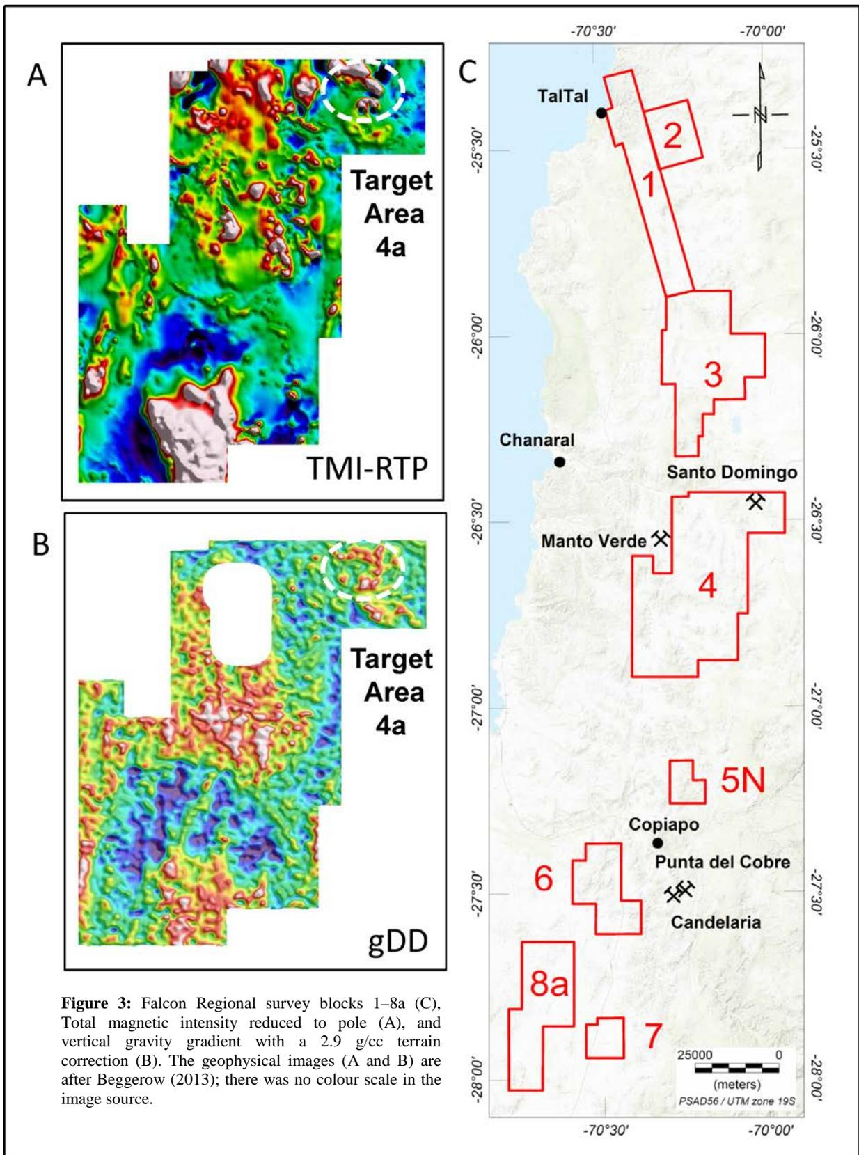
**Figure 3:** Falcon Regional survey blocks 1–8a (C), Total magnetic intensity reduced to pole (A), and vertical gravity gradient with a 2.9 g/cc terrain correction (B). The geophysical images (A and B) are after Beggerow (2013); there was no colour scale in the image source.
