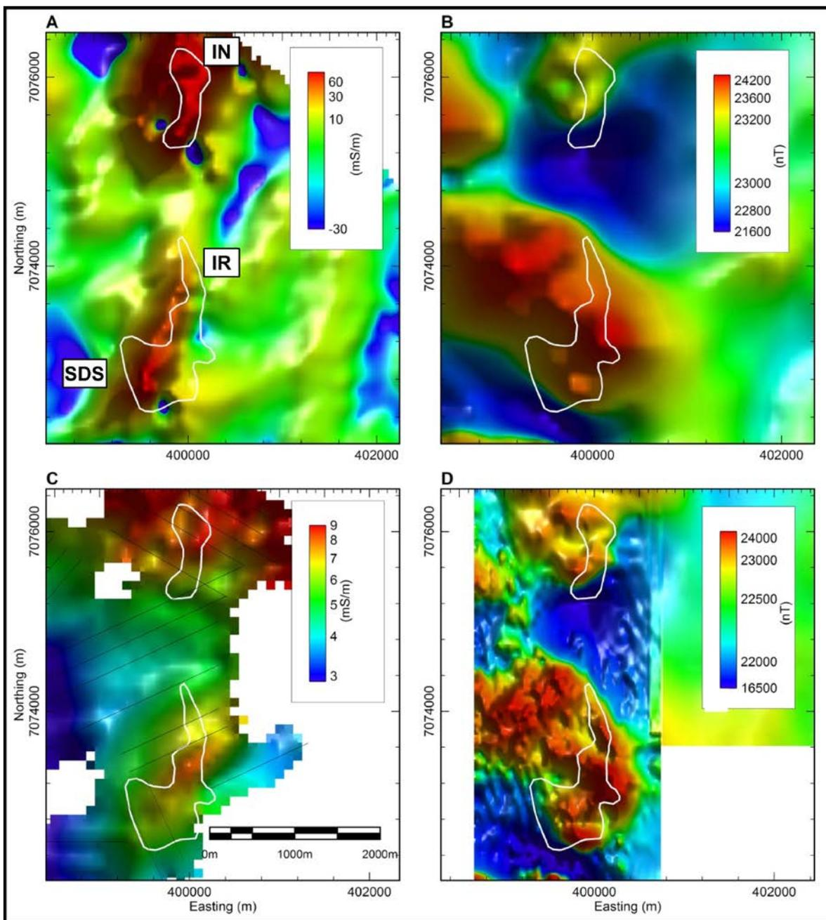
**Figure 11:** Section at 300 m below surface through 1D inversion of VTEM (A), TMI-RTP merged from VTEM and ZTEM surveys (B), Section at 300 m below surface through 1D inversion of surface 2007 TEM showing survey line locations (C), TMI-RTP merged from ground magnetic survey blocks.
