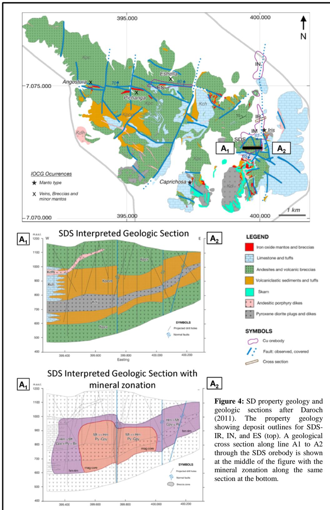
**Figure 4:** SD property geology and geologic sections after Daroch (2011). The property geology showing deposit outlines for SDS-IR, IN, and ES (top). A geological cross section along line A1 to A2 through the SDS orebody is shown at the middle of the figure with the mineral zonation along the same section at the bottom.
