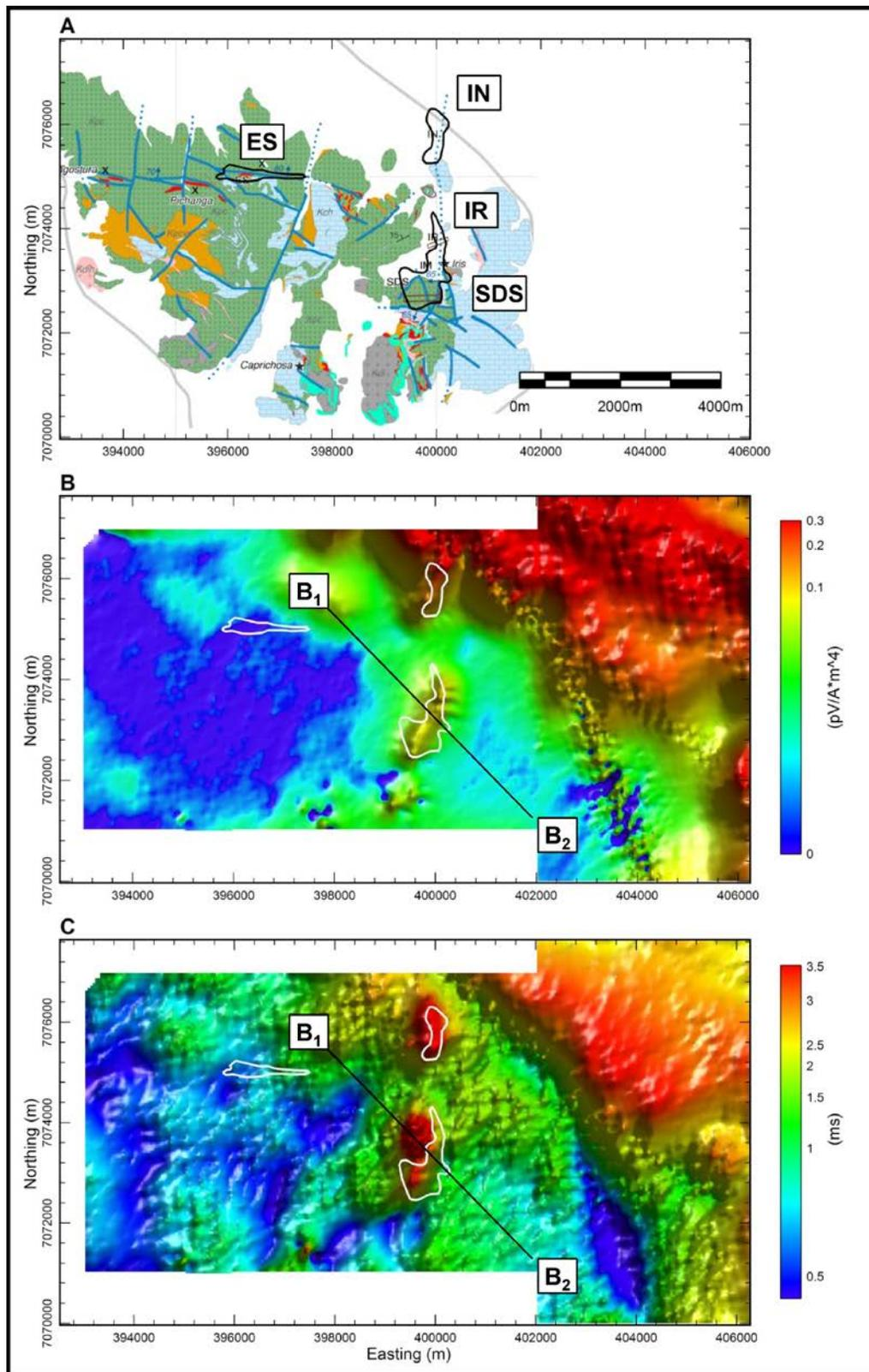
**Figure 7:** Property Geology after Daroch (2011) showing deposit outlines (A), VTEM dB/dt Z-coil amplitude at 3.521 ms (B), VTEM dB/dt Z-coil Adaptive Tau (noise limit 0.002 pV/(A\*m<sup>4</sup>)) (C). Black line represents the extent of section B<sub>1</sub> to B<sub>2</sub>.
