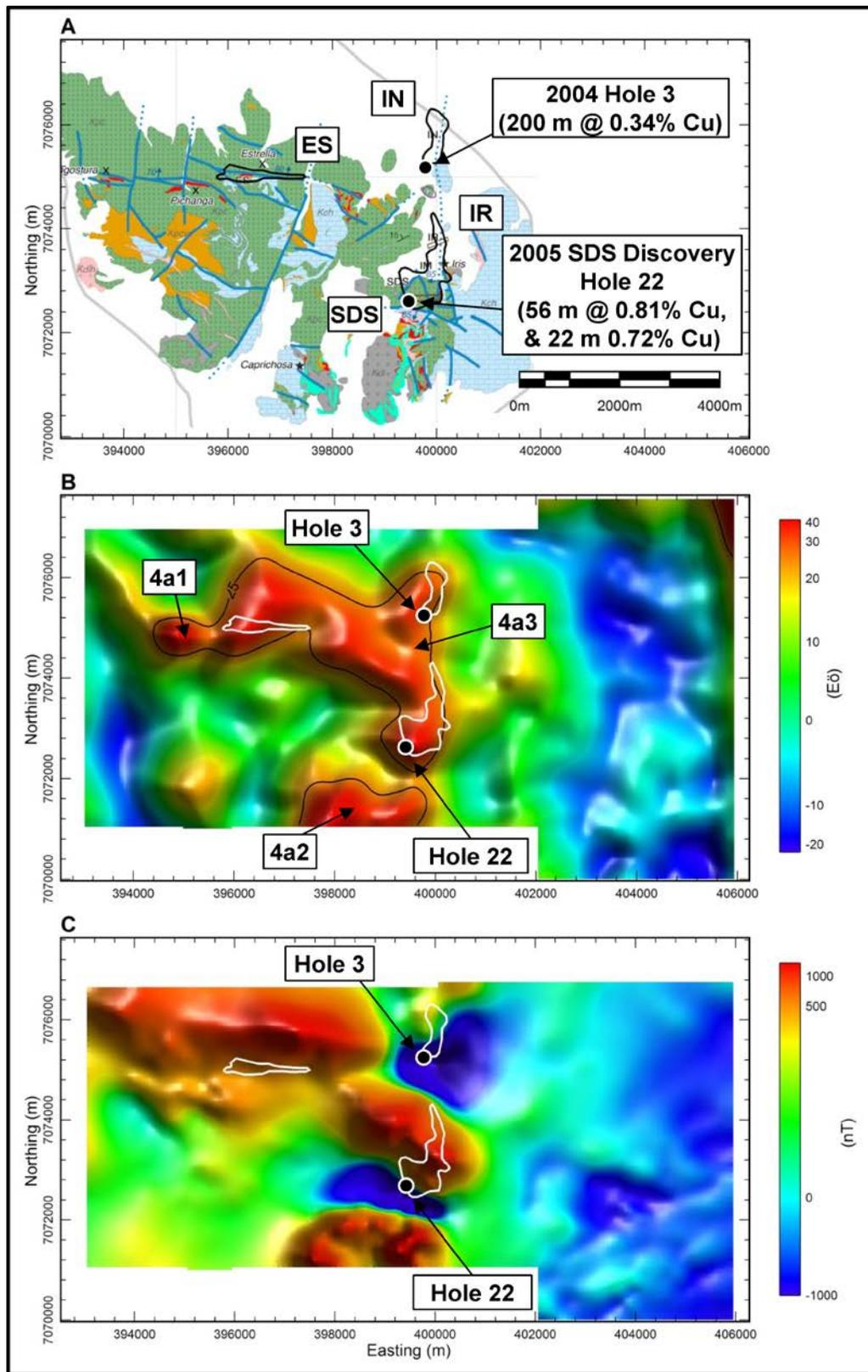
**Figure 6:** Property Geology after Daroch (2011) showing deposit outlines (A) and RC drill-holes, Falcon AGG gDD (2.90 g/cc terrain correction) with a contour at 25 Eö (B), and Falcon TMI-RTP (C).
