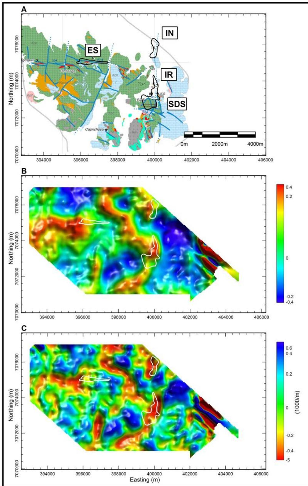
**Figure 8:** Property Geology after Daroch (2011) showing deposit outlines (A), ZTEM In-phase 75 Hz TPR (B), ZTEM In-phase 75 Hz DT (C).
