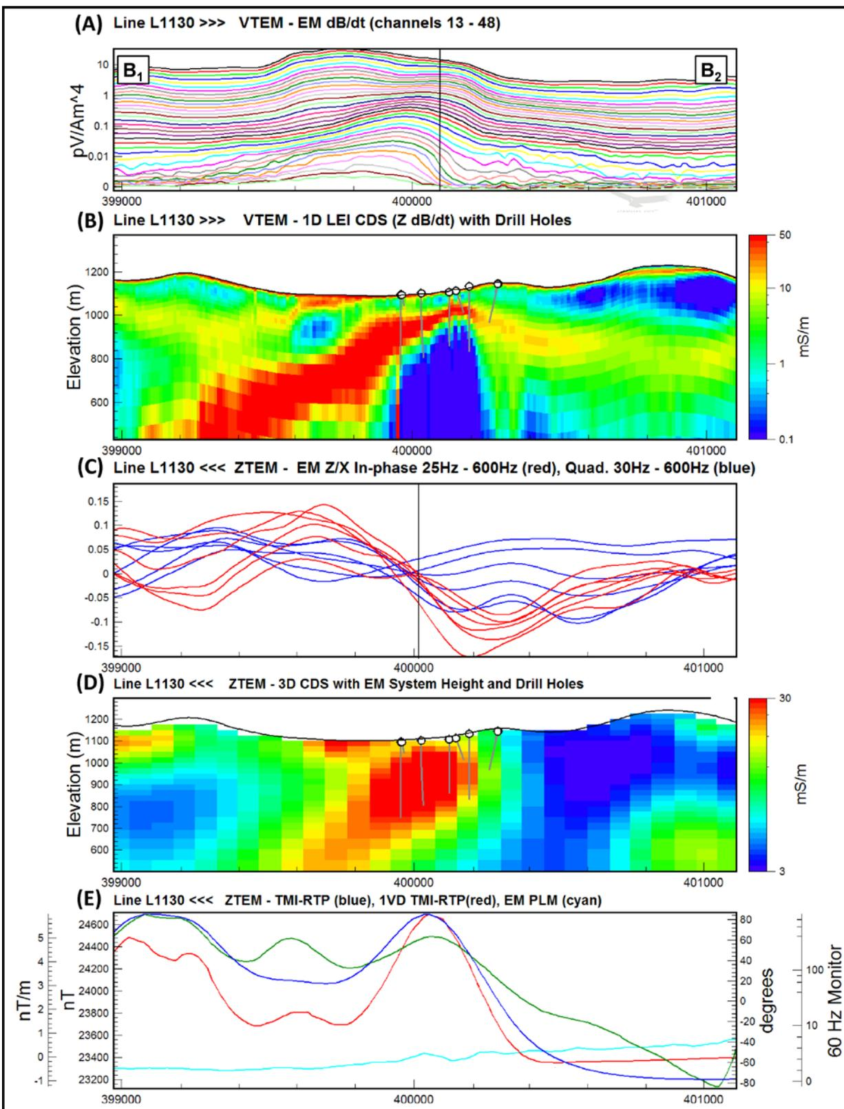
**Figure 10:** Stacked sections showing VTEM and ZTEM EM and magnetic results on L1130 over the SDS deposit. Centre of conductive source is indicated by a vertical black line. Section width corresponds to the black line between B<sub>1</sub> and B<sub>2</sub> in previous figures.
